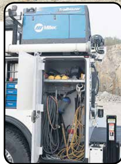
Miller Trailblazer 325 generator/welder has electronic fuel injection.
