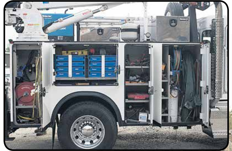
The 11-foot Autocrane Titan 60-Series service body has stainless steel hinges.
