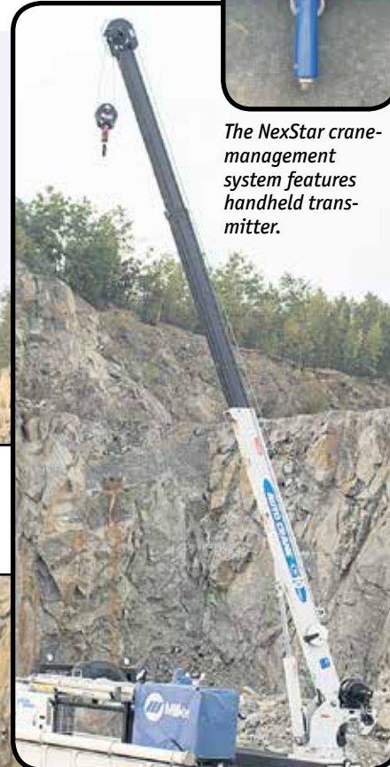
The Autocrane H10, 10,000-pound crane boasts a reach of 25 feet.
