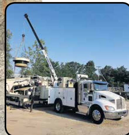
Autocrane H10 crane has 10,000-pound capacity.
