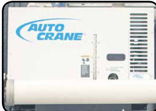
Autocrane AC40 hydraulically driven air compressor sits atop the left front compartment.
