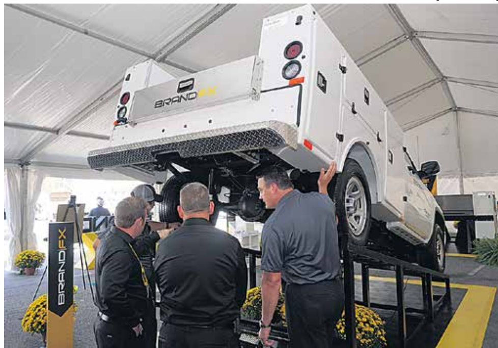
Daniels Sears of Drake-Scruggs Equipment, a BrandFX dealer in Springfield, Ill., goes over the features of BrandFX's UltimateFX composite body that includes a composite undercarriage on display at ICUEE 2017 in Louisville.
