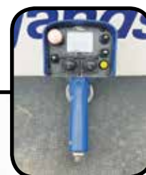
The NexStar crane-management system features handheld transmitter.
