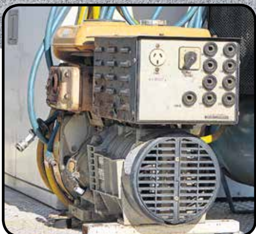
A 14-horse-power gas-powered Robin generator/welder provides on-site electricity and welding capacity.
