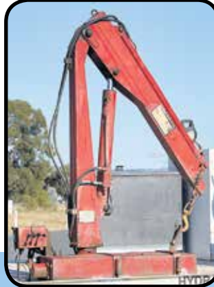
A basic 3000-pound Hyva crane with manual controls does the heavy lifting.
