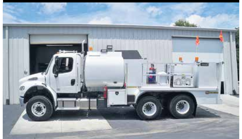
This lube truck by North Carolina's Taylor Pump & Lift features one 1,500-gallon fuel tank and four 125-gallon oil tanks, as well as tanks for waste, DEF and grease. Photo courtesy of Taylor Pump & Lift
