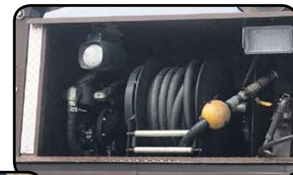
One of the hose reels is connected to an air-powered waste oil evacuation system connected to a 200-gallon tank.
