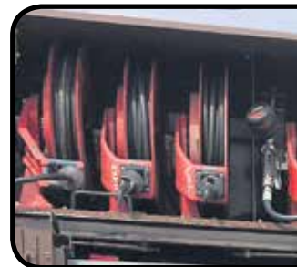
Individual hose reels dispense hydraulic oil, 15w-40 engine oil, 50-weight gear oil, 90-weight gear oil, extended-life antifreeze, or ethylene-glycol antifreeze.
