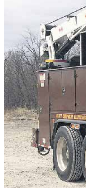
Randy Bostic's base truck is a 1989 Freightliner FLD112 powered by a 425-horsepower B-Model Cat engine
