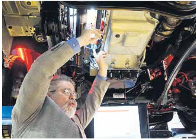
Chelsea marketing manager Jeff King shows how 249V Series PTO fits in tight space on a four-wheel-drive Ford truck.
