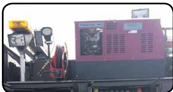
A Thermal Arc Predator Pro 300-amp welder rides on the top of his left side tool compartment, along with a second grease hose reel.
