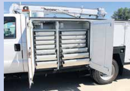
DuraLock drawers are non-abrasive and corrosion resistant, according to Maintainer. Photo courtesy of Maintainer Corporation of Iowa
