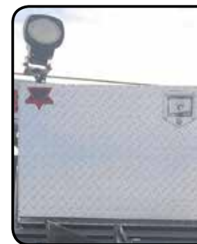
Chromed tool boxes are mounted to the top of the left side cabinets.
