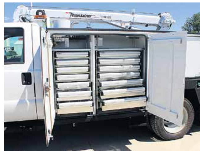
Maintainer's DuaLock aluminum drawer sets get their name from the drawer slide's locking feature, says the company website. Photo courtesy of Maintainer Corporation of Iowa
