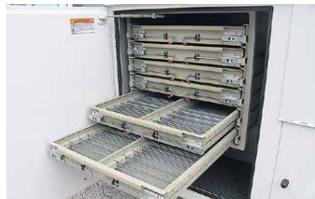
Knapheide's Plus 50 HD drawers are "rated at 250 pounds and have ball bearing guides to roll out and back smoothly," says the company website.
