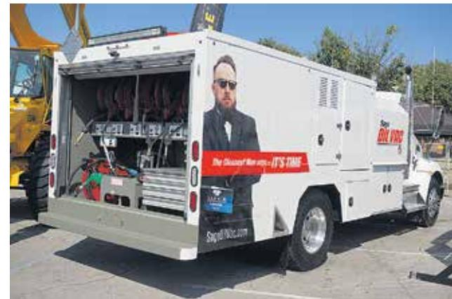
Sage Oil Vac's class 7 lube truck is mounted on a Volvo chassis.
