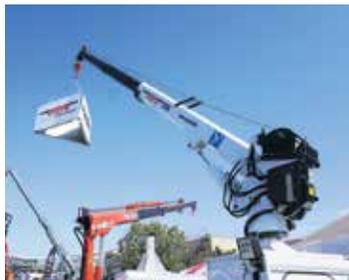
*Cobra 3800 electric-over-hydraulic crane and a smaller M150 Maxilift crane are mounted on a truck body at the Maxilift USA booth at ICUEE 2019.*
