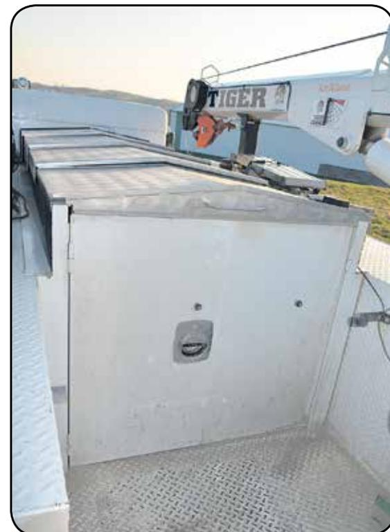
A sliding cover provides access to multiple 12-ton jack stands and other equipment.
