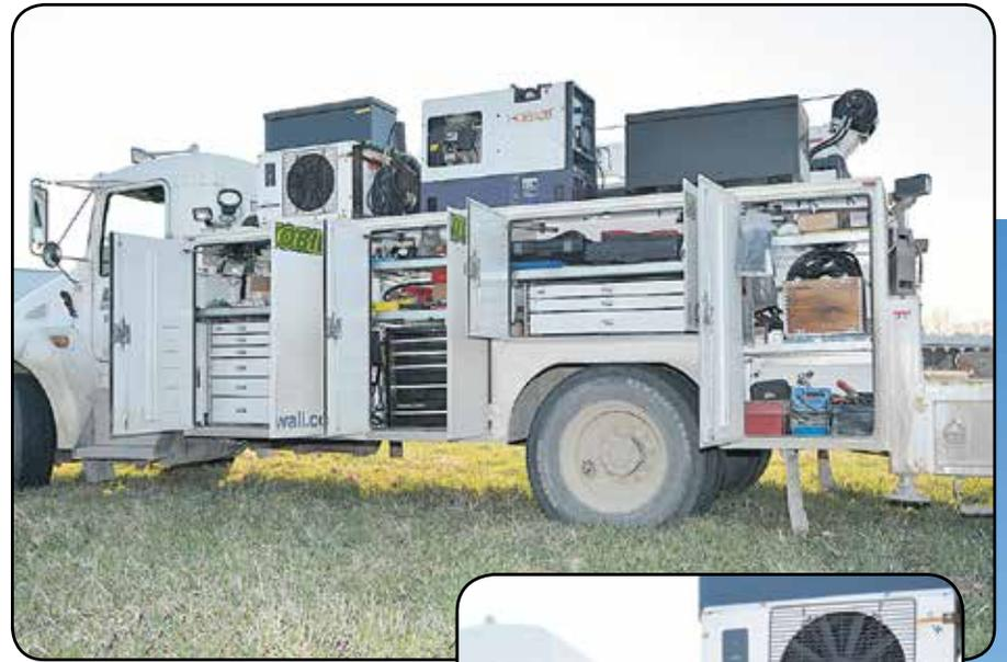
A 14-foot service body from Service Trucks International is equipped with three sets of Eagle Pro II tool chests.
