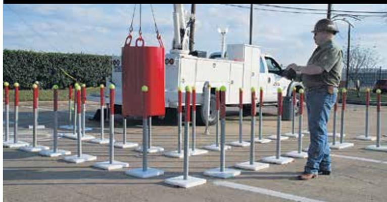
A candidate maneuvers the test load through the NCCCO's service truck crane operator practical exam in Houston in 2013. Photo courtesy of NCCCO
