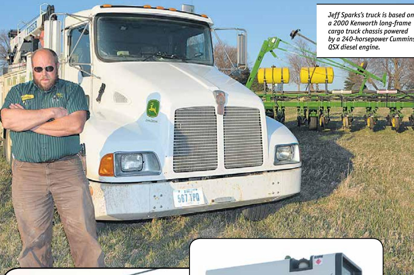
Jeff Sparks's truck is based on a 2000 Kenworth long-frame cargo truck chassis powered by a 240-horsepower Cummins QSX diesel engine.
